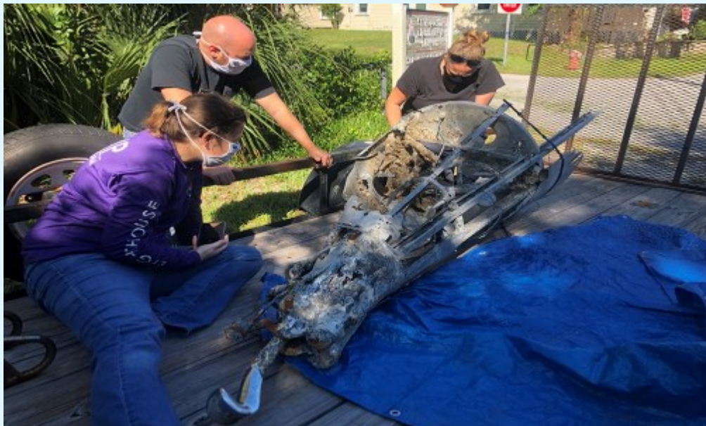
Photo Above: LAMP conservators Starr Cox, Dorothy Rowland, and Andrew Thomson inspect the tailpiece of a WWII era Grumman F4F Wildcat upon arrival at the museum in October of 2020. Note the prominent tail hook is still in place, used to capture the arresting cable during a carrier landing. (Copyright St. Augustine Lighthouse & Maritime Museum, Inc.)
