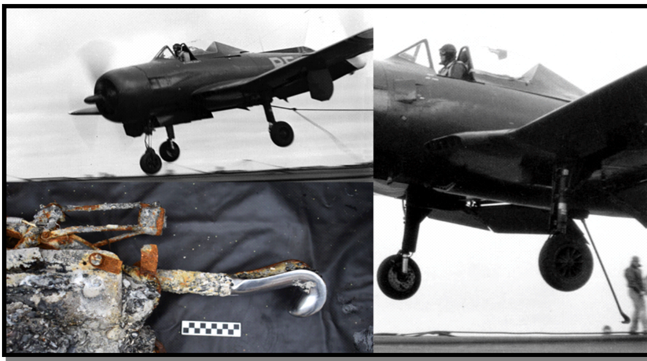
Figure 3 Upper left and right: WWII plane conducting landing operations on an aircraft carrier. Lower left: detail of the tail hook on the plane wreckage, note the excellent condition of the stainless steel on the hook's surface.
